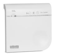
Wireless, wall mounted CO2 sensor measures the dioxide level in the room (PPM). Sensor works as a unit controller and indicates the current status by means of a multicolour LED. Up to 20 wireless devices can be connected to a single ventilation unit.
